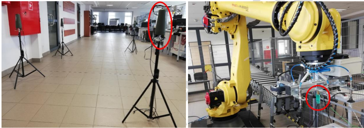
Fig. 4. The UWB beacons and the antenna module in the gripper of industrial robot during experiments.
