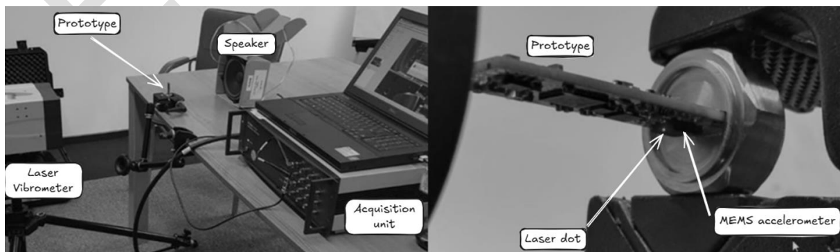
Fig. 1. Experiment set-up using Polytec PSV400 laser vibrometer – left-hand side picture. Laser beam pointed to the face of accelerometer in the direction of measurement – right-hand side picture.
