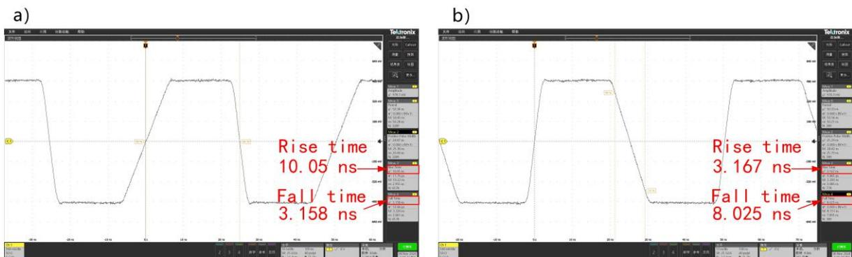
Fig. 14. Pulse edge time adjustment test a) The rise time is 10.05 ns the fall time is 3.158 ns. b) The rise time is 3.167 ns the fall time is 8.025 ns.
