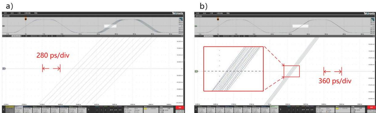
Fig. 12. Timing resolution test: a) pulse period with a 100 ps increment; b) pulse period with a 10 ps increment.
