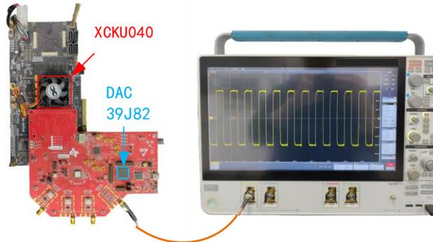
Fig. 10. Experimental test platform.
