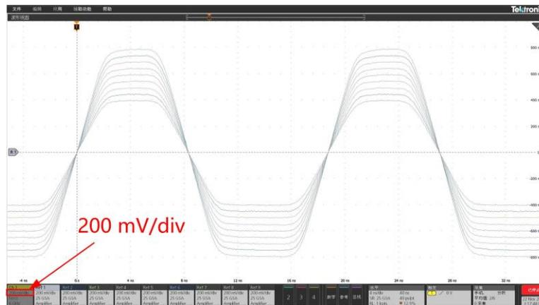
Fig. 15. Pulse peak-to-peak values in 100 mV increment.
