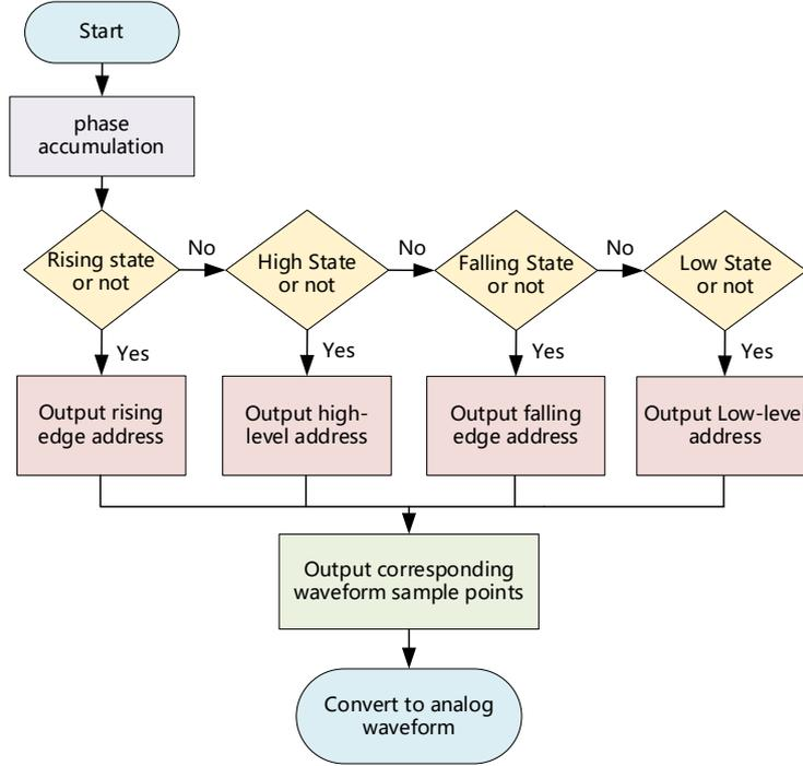
Fig. 4. Pulse waveform generation process.
