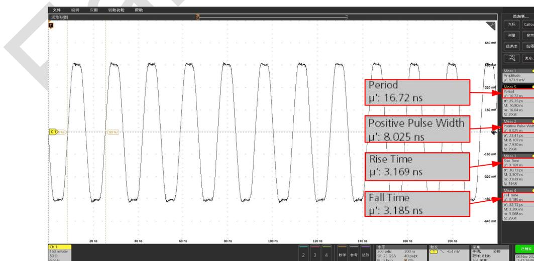
Fig. 11. Pulse waveform with a resolution of 100 ps, period of 16.7 ns, pulse width of 8 ns, rise time and fall time of 3.2 ns.
