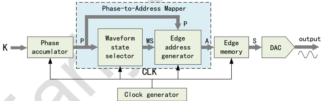
Fig. 3. Principle of pulse synthesis for feature-fitting.
