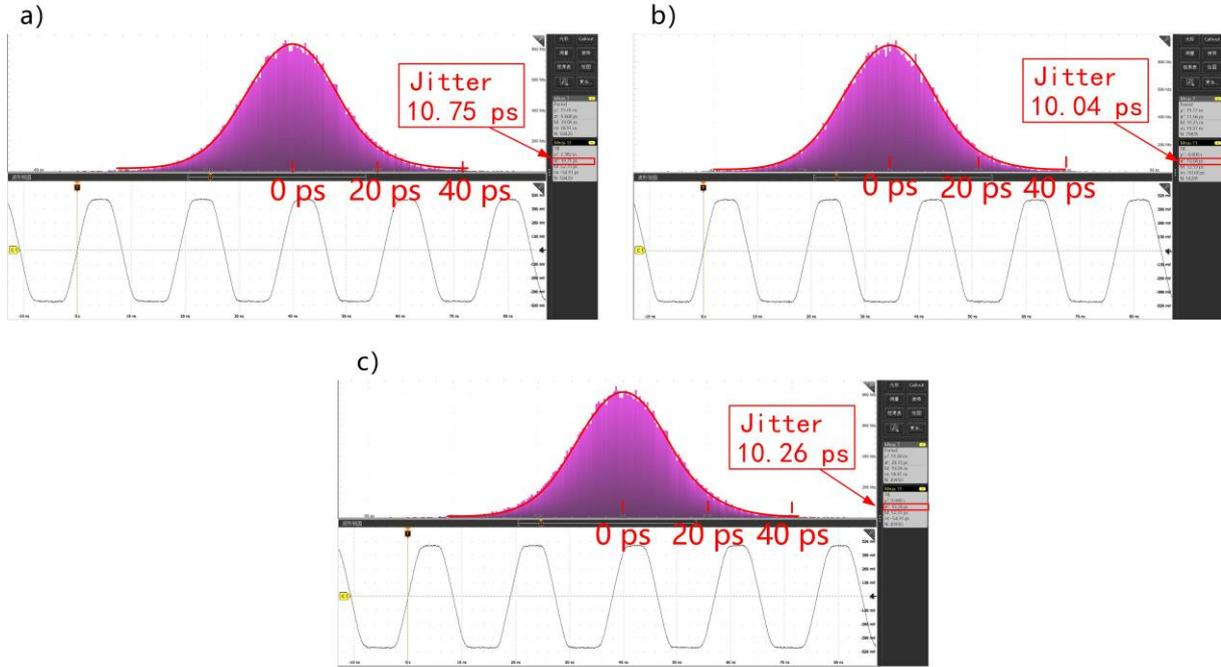
Fig. 16. Jitter test: a) of this scheme at 1 ns resolution, b) of this scheme at 100 ps resolution, c) normal DDS jitter at 1 ns resolution.
