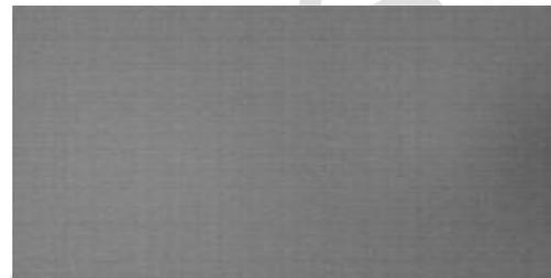
Fig. 8. Image of a large passive blackbody that fully fills imager's FOV.
