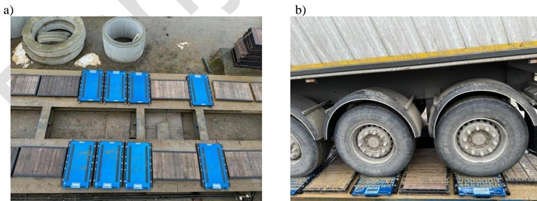
Fig. 1. Arrangement of the station for simultaneous weighing of vehicles on the platform scale and portable scales.
