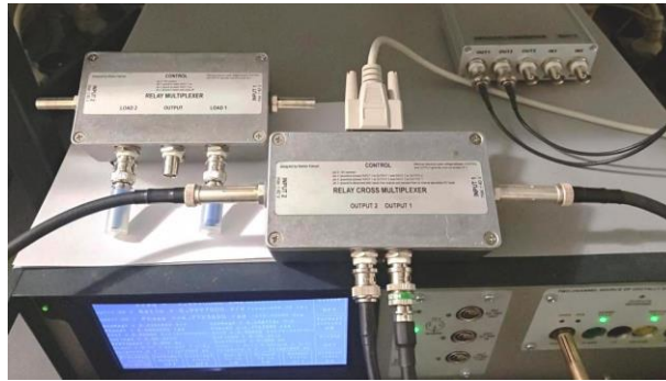
Fig. 3. Photograph of cross multiplexer. Old single output version of the MUX with external loads is visible on the top left.
