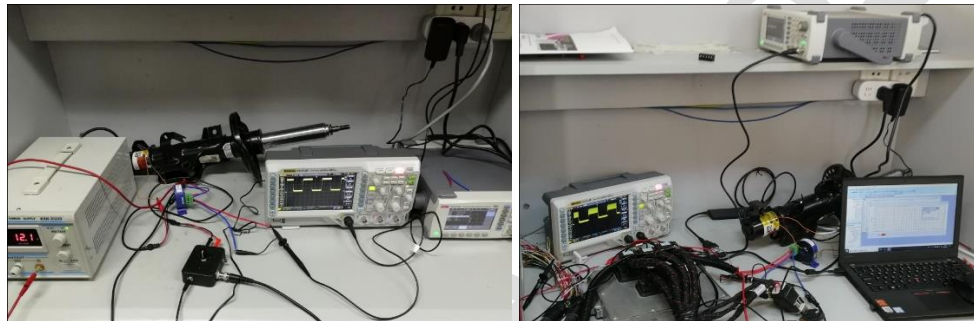
(a) Open-loop system. (b) Closed-loop system.
