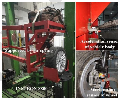
(a) McPherson test bench.
