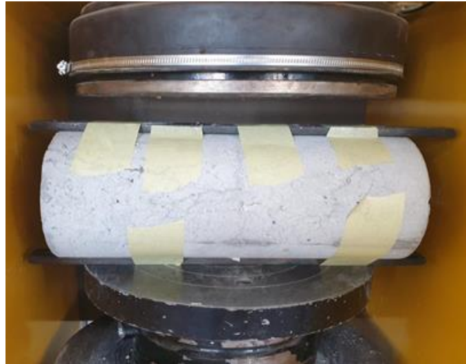
Fig. 11. A SFRC sample at time of Brazilian destructive test.
