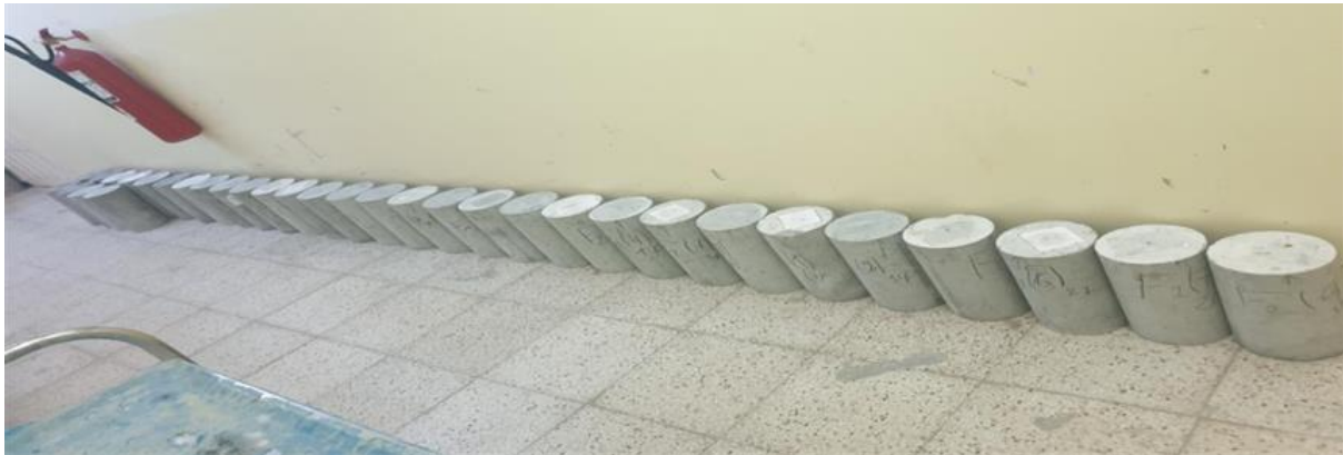
Fig. 10. Set of samples with random fiber distribution.
