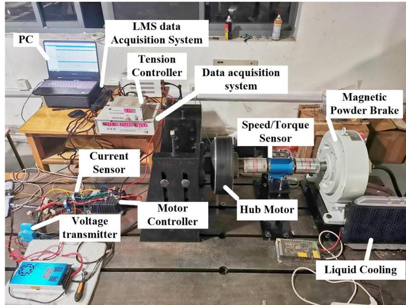
Fig. 7. Experimental platform for parameter identification of hub motor.
