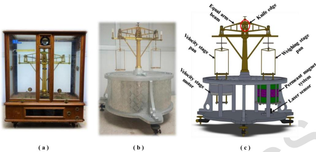
Fig. 1. The KB illustration: (a) Two-pan equal-arm balance before modification, (b) Modified KB and (c) 3D CAD model of NIS's KB.
