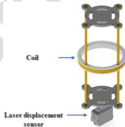
Fig. 5. Suspension system of the coil.
