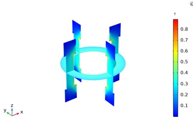
Fig. 6. Distribution of the magnetic flux in the air gap.
