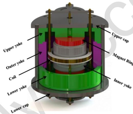
Fig. 3. Structure of the NIS permanent magnet assembly.
