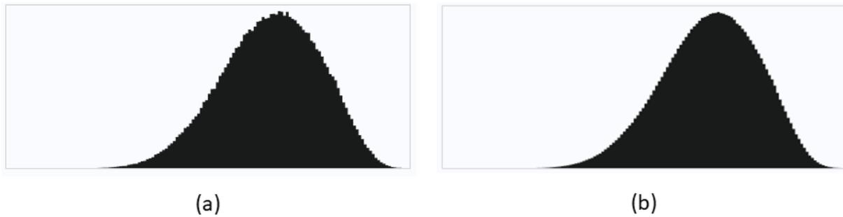
Fig. A.2. Histogram of element quality (a) with the number of mesh elements 1115336 (b) with the number of mesh elements 7558093.
