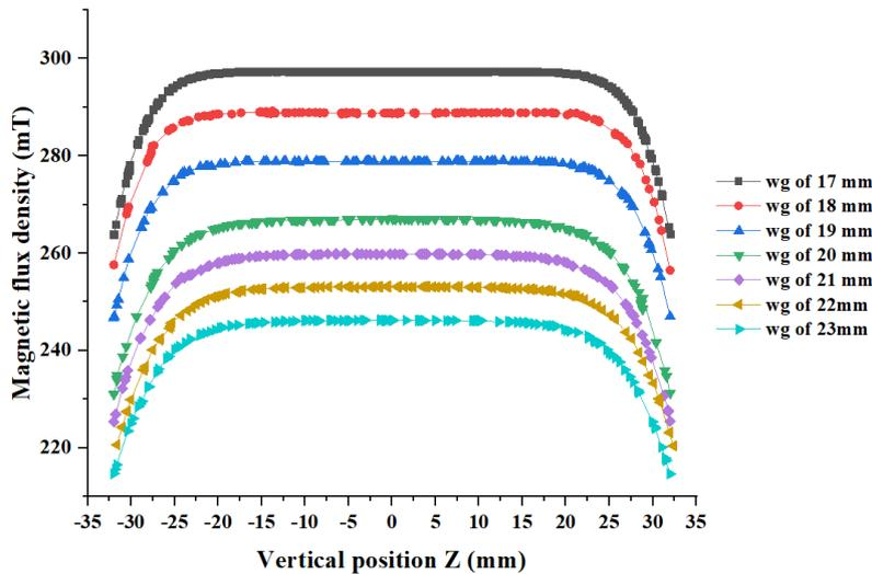
Fig. 9. Magnetic flux density at the vertical position Z for different air gap widths.
