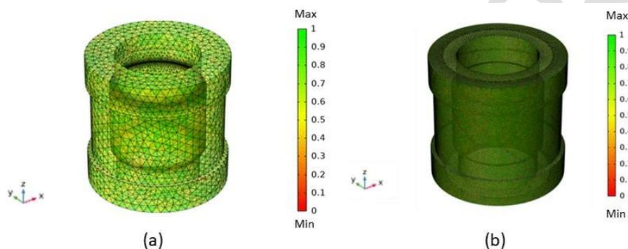
Fig. A.3. Elements quality of air gap domain (a) elements with low quality (b) elements with high quality.
