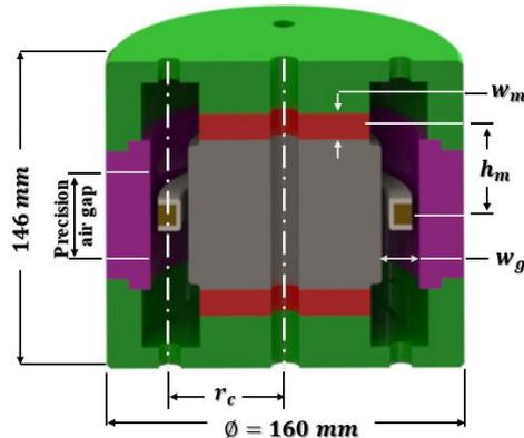
Fig. 4. Cross-section view of the NIS magnet system.
