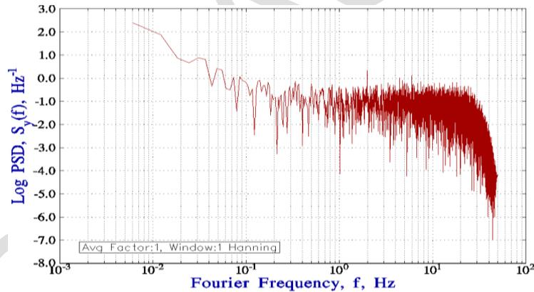
Fig. 5. PSD for the comparison 10 T $\Omega$  MI:100 T $\Omega$  Gdl with positive polarity at 1000 V, from 0 Hz to 50 Hz.
