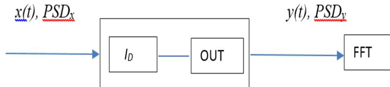
Fig. 4. Setup to evaluate the noises at the detector whose output circuit is connected to a FFT analyser.
