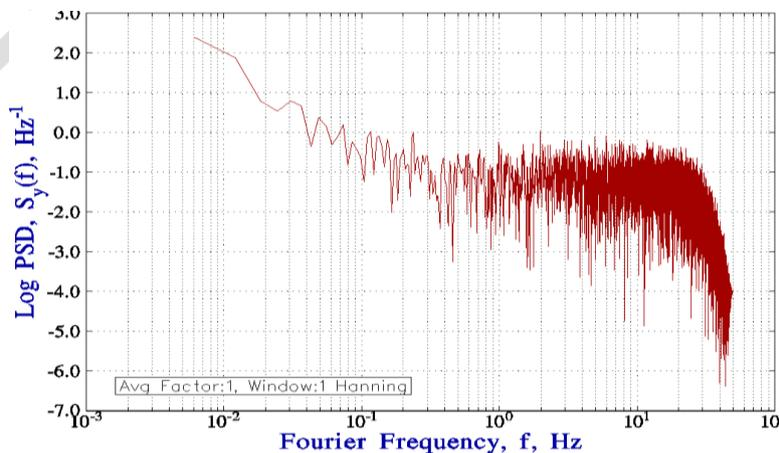
Fig. 6. PSD for the comparison 10 T $\Omega$  MI:100 T $\Omega$  Gdl with negative polarity at 1000 V, from 0 Hz to 50 Hz.
