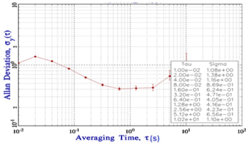
Fig. 7. AD for the comparison 10 TΩ MI:100 TΩ Gdl with positive polarity at 1000 V.
