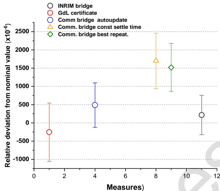
Fig. 12. Compatibility check among the measurements with the commercial bridge, with the INRIM DSB bridge and the value of the Guildline certificate of the 100 T $\Omega$  resistor. The uncertainty bars correspond to the expanded uncertainty at 95.5 % confidence level.
