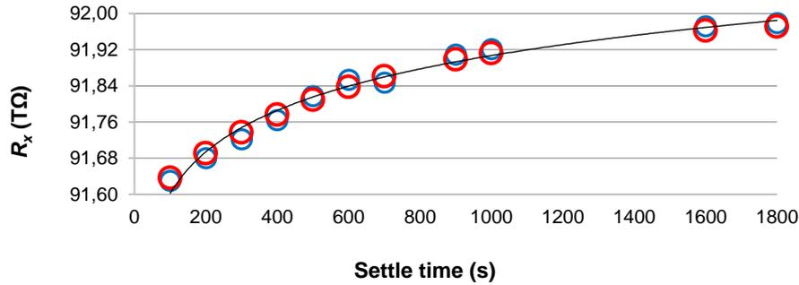
Fig. 3.  $R_x$  value as function of the settle time for the 10 TΩ-100 TΩ ratio at 1000 V. In blue, the measured values while in red those estimated with the (2) are respectively shown.
