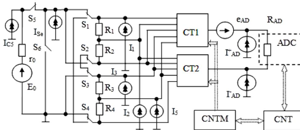
Fig. 1. Code-controlled resistive divider with automatic zero correction during ADC testing.
