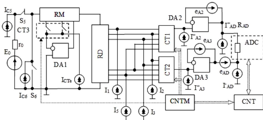
Fig. 2. Improved device for operative metrological monitoring of measuring channels of cyber-physical systems.
