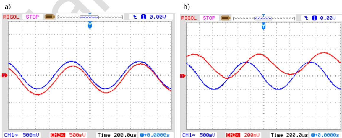
Fig. 8. Graphs of signals  $x(t)$  and  $z(t)$ : a)  $f_x = f_y = 1\text{kHz}$ ;  $\varphi_0 = 4,1^\circ$ ; b)  $f_x = f_y = 1\text{kHz}$ ;  $\varphi_0 = 71,5^\circ$ ; broadband noise  $N(0,100 \text{ mV})$ .
