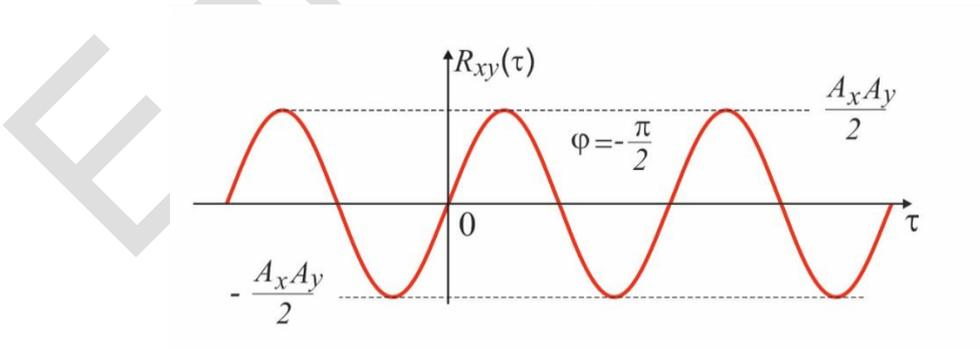
Fig. 5. Correlation function  $R_{xy}(\tau)$  for  $\varphi = -\frac{\pi}{2}$ .
