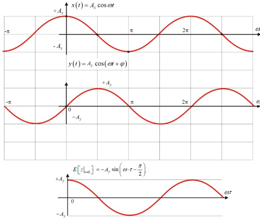
Fig. 1. Models of signals for  $\varphi_p = 0^\circ$  and  $\varphi = -90^\circ$  and characteristic  $E[z|x=0]$  for  $\varphi = -90^\circ$ .
