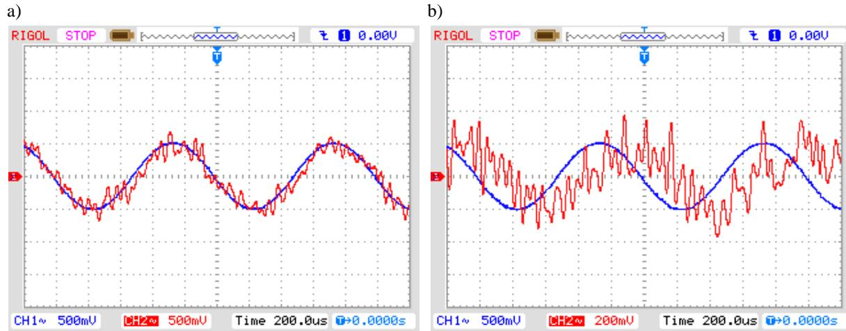
Fig. 7. Waveforms of signals  $x(t)$  and  $z(t)$ : a)  $f_x = f_y = 1\text{kHz}$ ;  $\varphi_0 = 4,1^\circ$ ; b)  $f_x = f_y = 1\text{kHz}$ ;  $\varphi_0 = 71,5^\circ$ ; broadband noise  $N(0,100 \text{ mV})$
