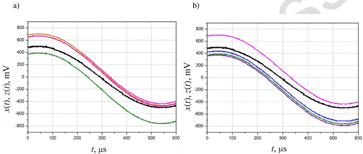
Fig. 9. Waveforms of signals  $x(t)$  (black) and  $z(t)$  (coloured):  $f_x = f_y = 1 \text{ kHz}$ ,  $\varphi_0 = 0^\circ$ ; subsequent averaged characteristics  $z(t + \tau)|_{x(t)=0}$  with positive values of low-frequency interference (a) and negative values (b).
