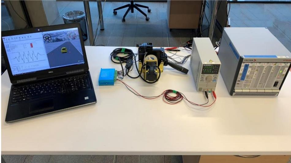
Fig. 6. Steering wheel angle sensor test bench.
