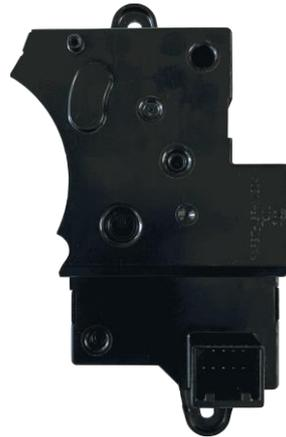
Fig. 2. Example of a steering wheel angle sensor (SAS).
