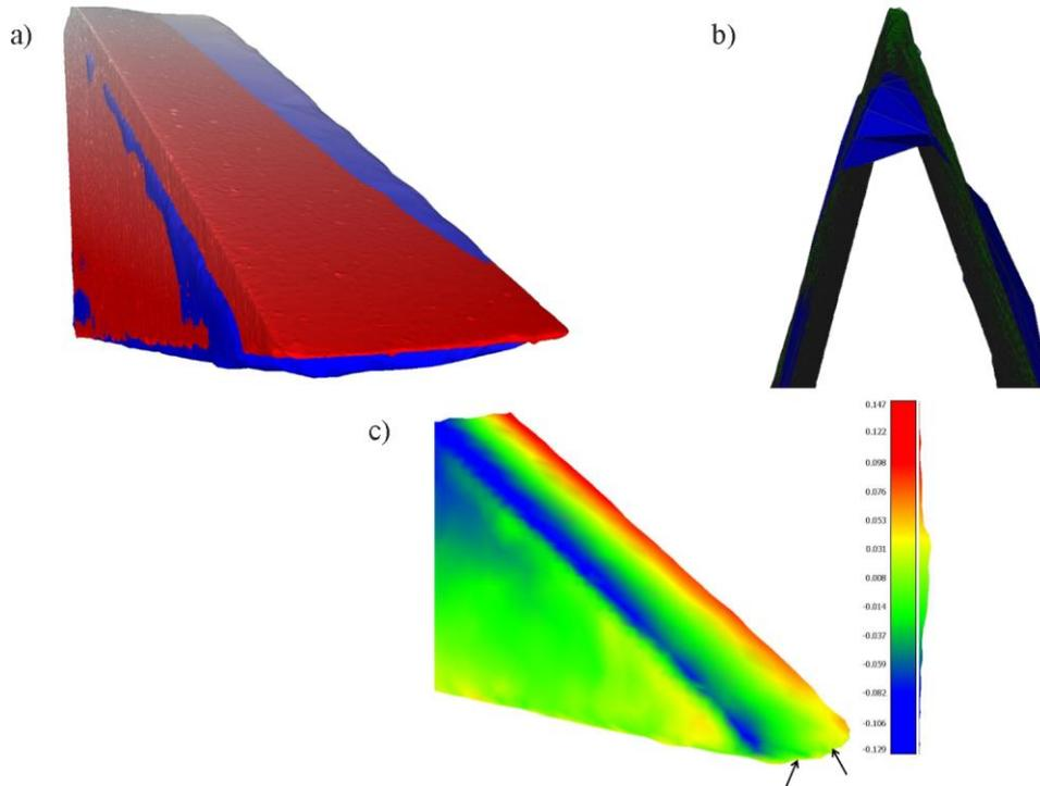
Fig. 4. a) registration/superposition of the mesh recorded from the microCT image and the CS3600 camera; b) detail of the superposition on a region of interest; c) colored map representation of distance calculated by projection of the camera mesh vertex on microCT mesh faces. Black arrows: the distance values of interest.
