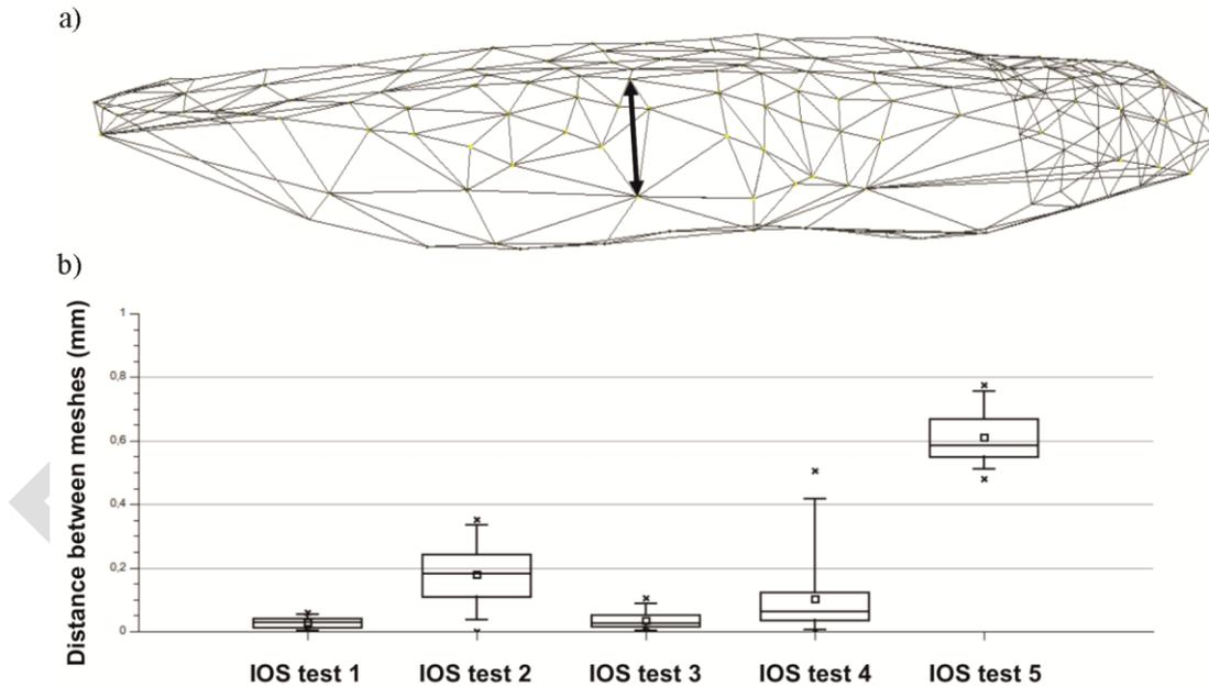
Fig. 5. a) scheme of distance calculation between two faces with IOS mesh; b) Distance between mesh for the microCT and the CS3600 camera (IOS) for 5 different acquisitions (test 1-5) Box plot: rectangle: 25% to 75%.
