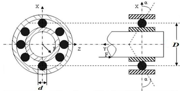
Fig. 2. Geometric characteristic of a bearing.
