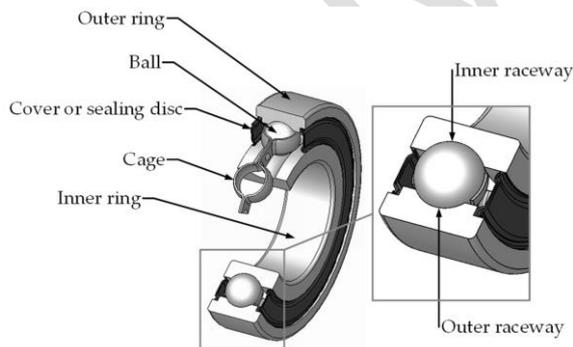
Fig. 1. Diagram of the construction of a rolling bearing [11].
