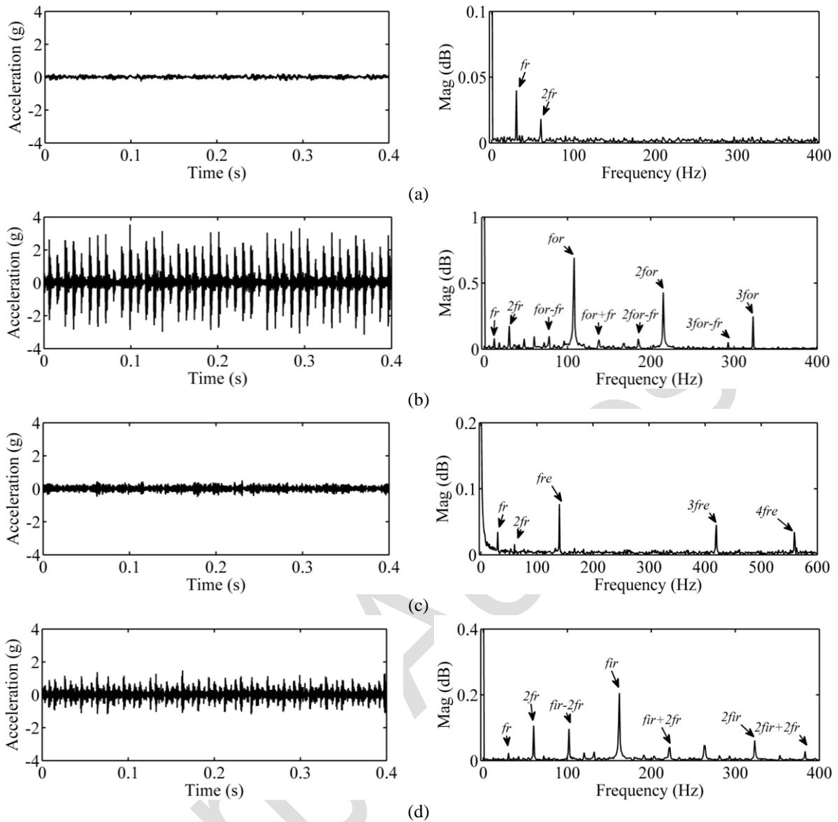
Fig. 4. Vibratory signatures and spectral envelope analysis. (a): healthy bearing. (b): bearing with an outer race fault. (c): bearing with a rolling element fault. (d): bearing with an inner race fault.
