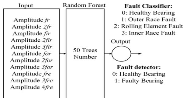
Fig. 6. Schematic diagram of RF.
