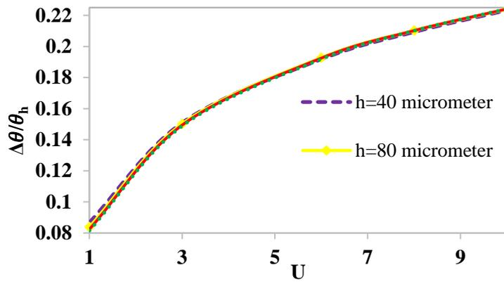
Fig. 6. The effects of bottom cavity height  $h$  on the sensor's temperature difference ( $\frac{\Delta\theta}{\theta_h}$ ).
