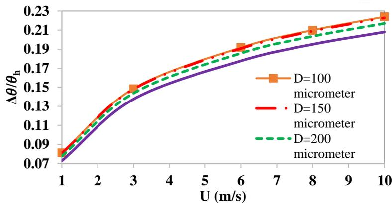
Fig. 7. The effects of distance between the heater and the sensing elements on the sensor's temperature difference ( $\frac{\Delta\theta}{\theta_h}$ ).
