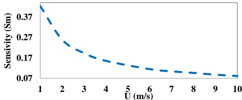
Fig. 4. Thermo-resistive micro calorimetric flow sensor sensitivity.
