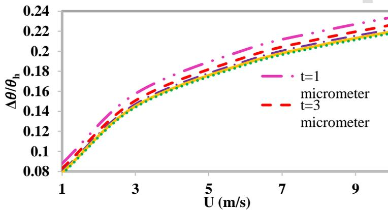
Fig. 5. The effect of thin-film thickness on Thermo-resistive micro calorimetric flow sensor  $\frac{\Delta\theta}{\theta_h}$ .
