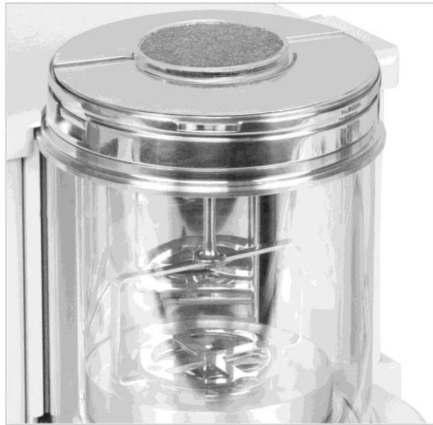
Fig. 8. Balance during the measurement of magnetic susceptibility.
