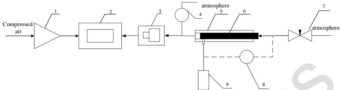
Fig. 3. Diagram of the differential pressure compensation principle for ventilation rate measurement based on a digital thermal flowmeter: 1. gas pressure regulator; 2. negative pressure generator; 3. tobacco special standard constant flow hole; 4. differential pressure sensor 1; 5. special fixture; 6. tobacco special ventilation rate standard rod; 7. needle valve; 8. differential pressure sensor 2; 9. digital thermal flow sensor.
