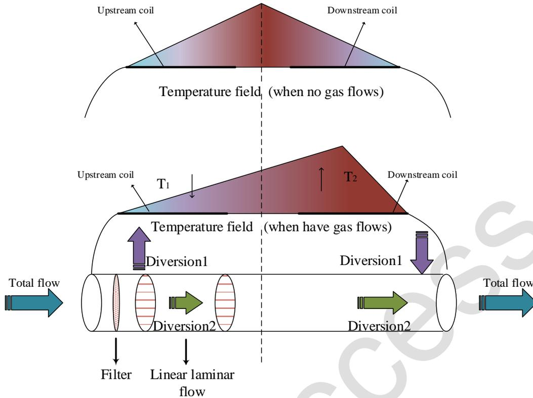
Fig. 2. Measuring principle of digital thermal flowmeter.
