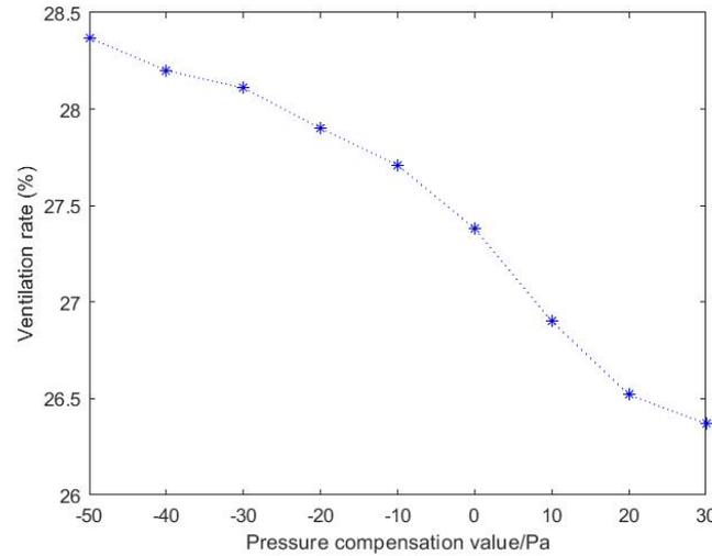
Fig. 4. Ventilation rate curve under different pressure differences.
